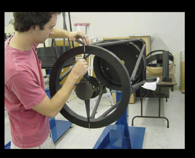
16" prototype composite optical tube assembly being assembled in Tucson
